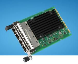
Quad-port Gigabit Ethernet network adapter for OCP NIC 3.0 specification designed with performance enhancing features and power management technologies
