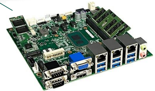
NexAIoT Controller RCB600 Powered by Intel® Core™ i7 processor based industrial PC
