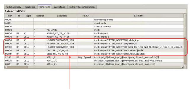
The HSSI refclk goes through HSSI refclk divder and core clock network via CLKCTRL
