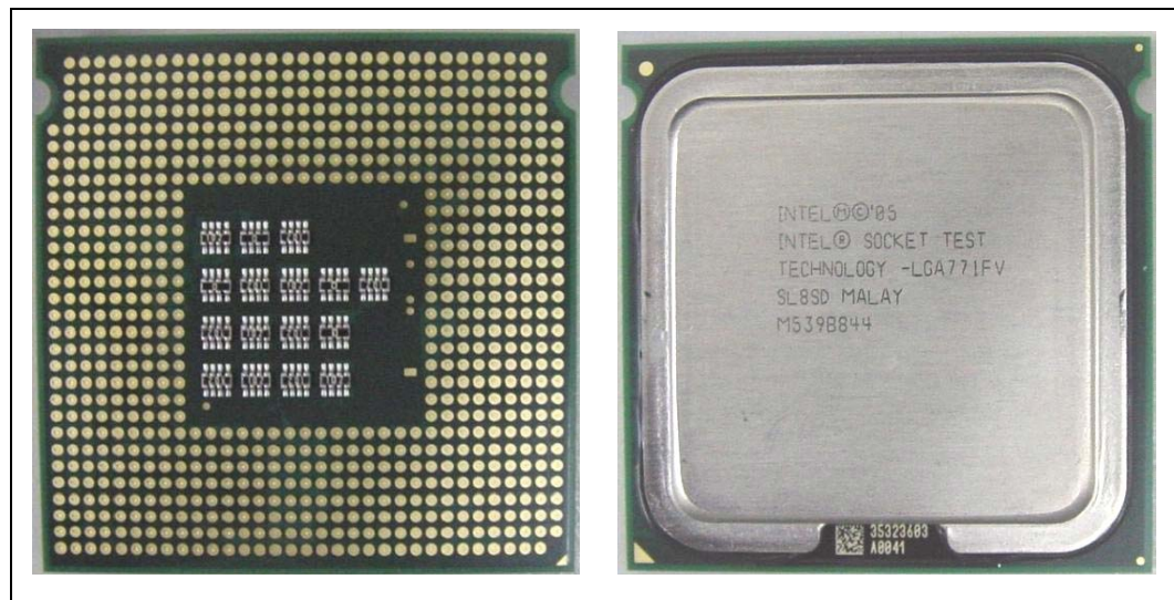
Figure 1-1. Intel® Socket Test Technology for the LGA771 Socket-Test Chip JM8FKZLVA
